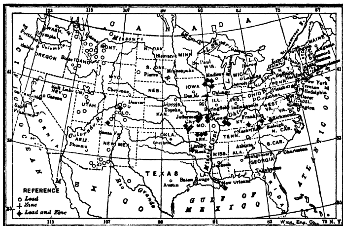
FIG. 188.—Map showing distribution of lead and zinc ores in the United States. (Adapted from Ransome, Min. Mag. , X.)
